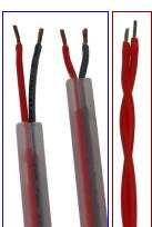
Then position the 4" piece of Shrink Tubing centered over the wrapped connections completely covering the stripped section. Use the Heat Gun or Blowtorch to shrink the tubing\*.
