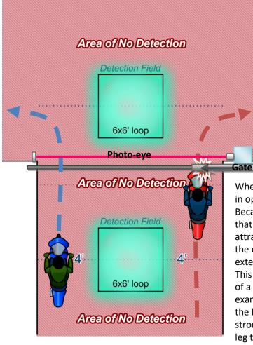
Many installers are taught that if a loop's detection height or field will extend around the loop in all directions. This causes installers to install loops up to 4 - 4.5ft away from the curbs or side of the roadway.
