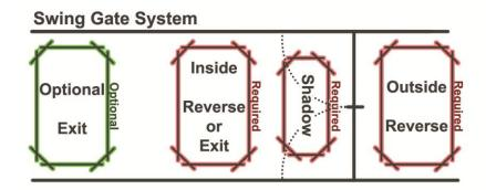
If space permits you may want to install an additional Exit Loop further down the driveway so that the gate will be open by the time the vehicle reaches the gate.
