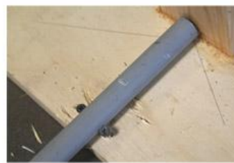
1/2" Schedule 40 Rigid PVC Conduit after the third drop.
