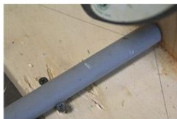
1/2" Schedule 40 Rigid PVC Conduit after the first drop.
