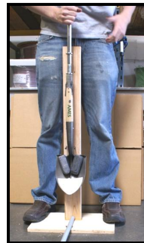
Example of Drop Height with PVC conduit in position
