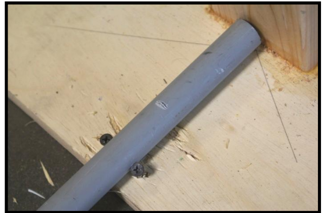
½" Schedule 40 Rigid PVC Conduit after the third drop.
