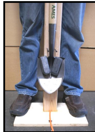
Example of Drop Height with XLPE wire in position
