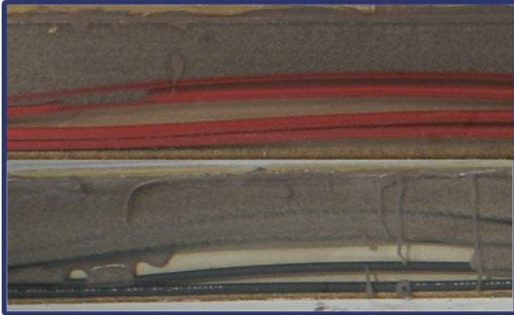
Figure 1 - Air Pockets in 1/8" Groove.
