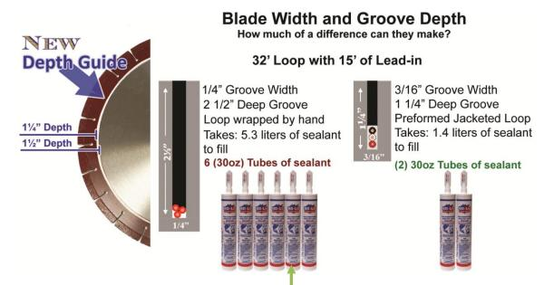
Use a 3/16" blade to save 25% in sealant (vs. a 1/4" blade).
