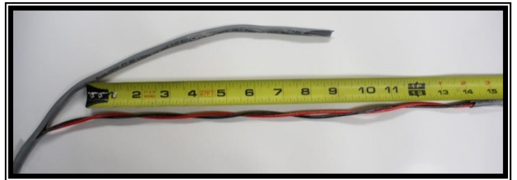
*Inside of Twisted Pair (7 twists per foot)
