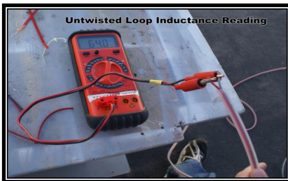
Figure 1 Inductance Reading of untwisted Loop 64.0 \mu\text{H}
