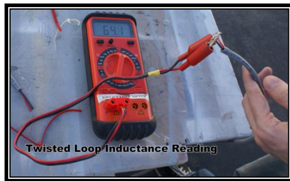
Figure 2 Inductance Reading of Twisted Pair Loop 64.1 \mu\text{H}
