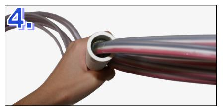
You might want to add a 1" to 1/2" reducer coupler that will allow you to run the lead-in through 1/2" PVC conduit from the yoke to the operator.
